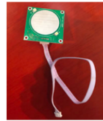
capacitive touch buttons + external cables (can be put under 3mm glass plate)
