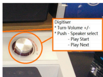
external Press and Turn button + external cable
