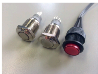
external press-buttons + external cable
