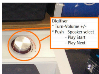
external Press and Turn button + external cable
