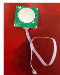
capacitive touch buttons + external cables (can be put under 3mm glass plate)
