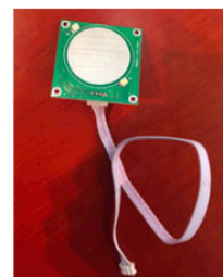
capacitive touch buttons + external cables (can be put under 3mm glass plate)
