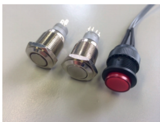
external press-buttons + external cable
