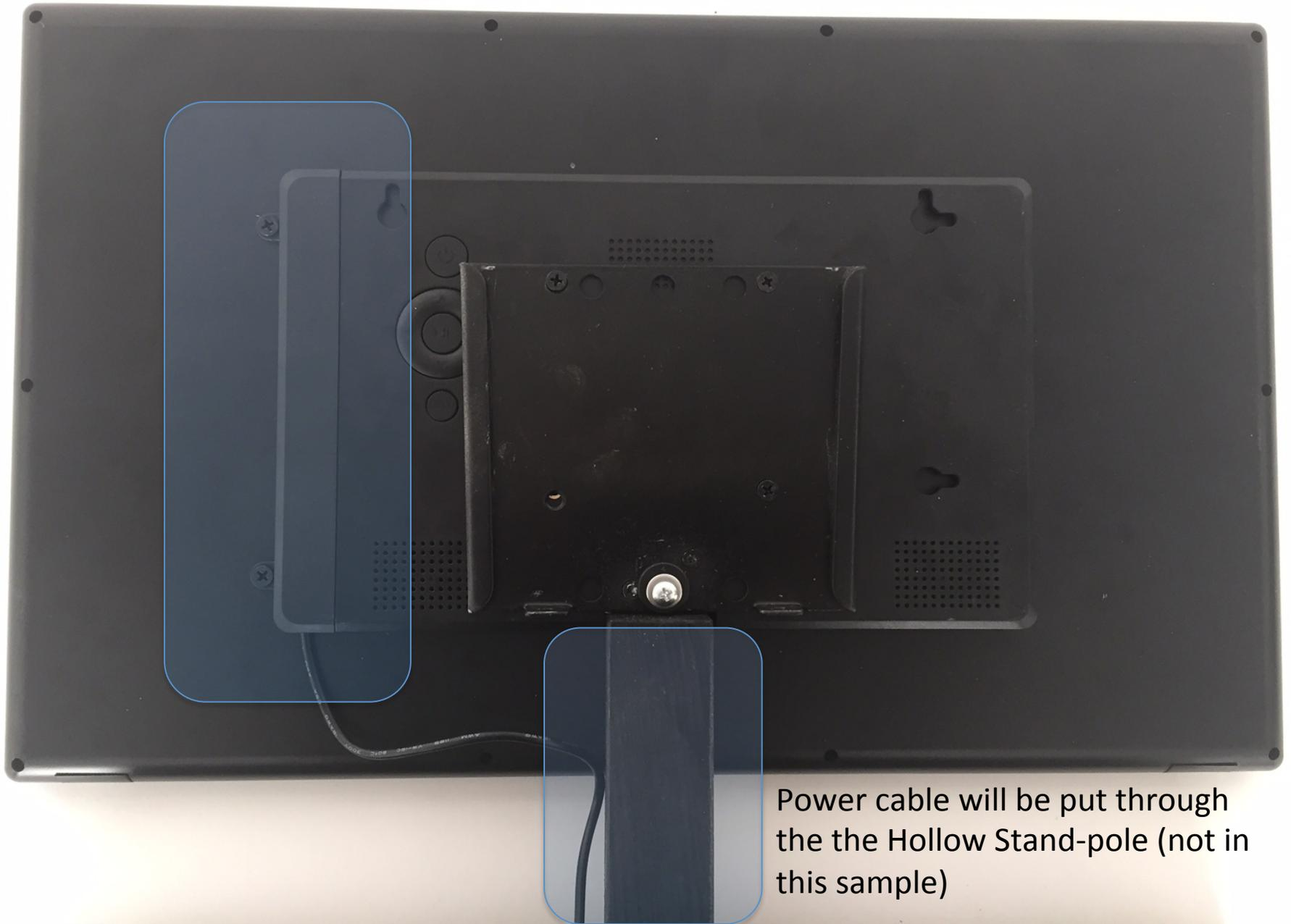
Power cable will be put through the the Hollow Stand-pole (not in this sample)
