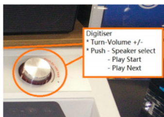
external Press and Turn button + external cable
