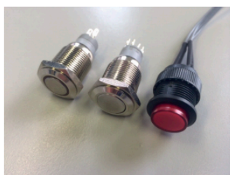
external press-buttons + external cable
